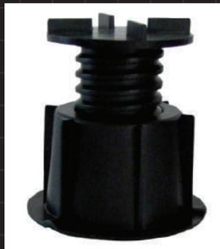
various adjustable sizes from 20mm to 65mm. The underside of the base is smooth with no sharp edges that may damage the membrane. The width of the base is also sufficient to spread the load of both the dead and live loads transferred onto the membrane through the Deck Jak®. The base also incorporates water egress channels to allow any build up of water within the Deck Jak® to disperse.
