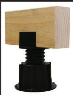
are spaced to accept 45mm timber and are grooved to allow easy penetration of fixing nails or screws. One 30mm galv or stainless (as required) nail or screw should be used on each side of the Timber Top® Spacers of Timber Tops® should be in accordance with NZS3604 2011 joist spans.(see section 7) to suit the size of the timber being used.
