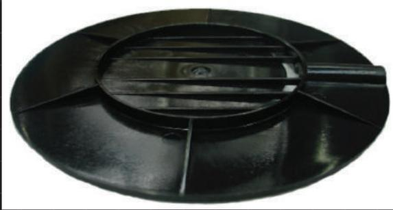
Utilised in some specific conditions, whilst not a requirement of the system in general, merit has been found in providing a larger footprint in the instance of a heavy dead load. The Base Plate has also been designed with sloping splines to allow for an increase in slope of the substrate by 2°. This allows Joist Jaks™ to be used on decks or substrates with a 4° fall.
